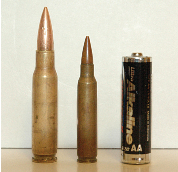
Figure 9-9. 7.62 vs 5.56 military bullets. Reproduced from: http://en.wikipedia.org/wiki/File:7.62x51_5.56x45.JPG
